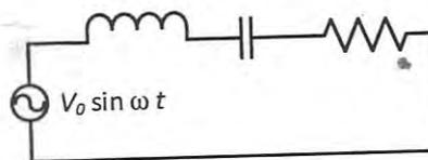
[A] At  $\omega \gg 10^6 \text{ rad. s}^{-1}$ , the circuit behaves like a capacitor
