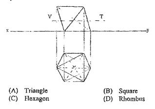
123. A tetrahedron resting on HP as shown is cut by a cutting plane. What is the true shape of section?
